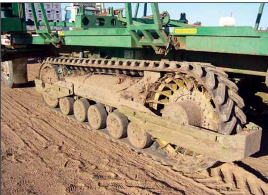
The 280-lb. cast drive wheels serve as the main drive component for a track-driven produce harvesting machine.
